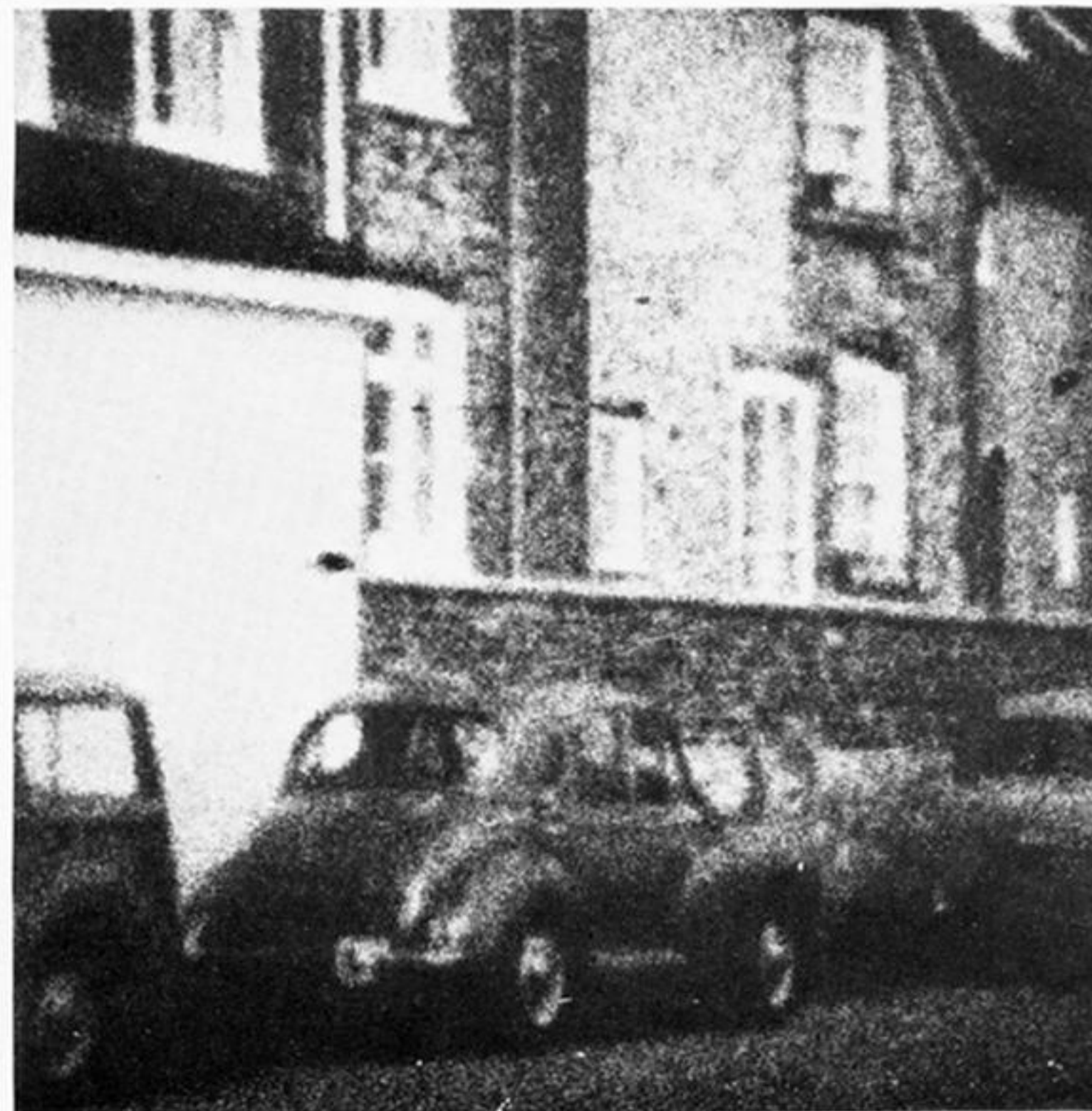
FIGURE 18. Photograph of image detail on screen of XX 1060, corresponding to different scene illumination levels, with an exposure time of 0.2 s. (a) 0.03 mlx (very dark sky, no moon), (b) 0.1 mlx, (c) 0.3 mlx, (d) 1 mlx (approx. starlight: no cloud, no moon), (e) 2 mlx, (f) 50 mlx (approx. full moon).
