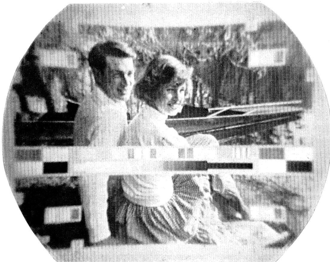
FIGURE 22. Photograph of the image on the viewing screen of an experimental channel image intensifier tube.
